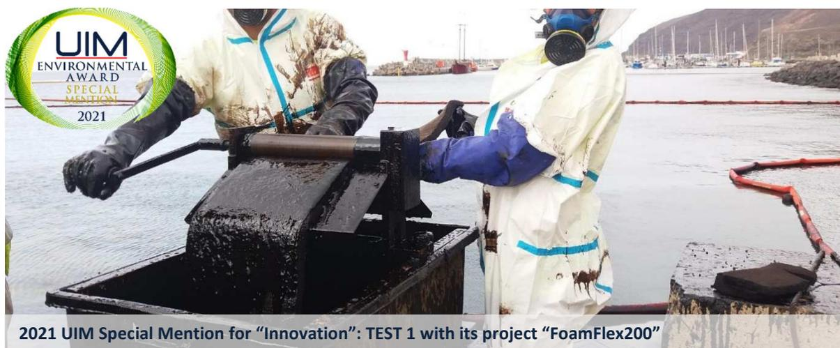
The recipient of the 2021 UIM Special Mention for Innovation is Italian company Test1 for its project FoamFlex200, a selective sponge able to absorb only hydrocarbons for about 30 times its own weight, while repelling water.
